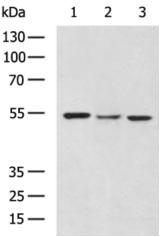
Gel: 8%SDS-PAGE, Lysate: 40 µg; Lane 1-3: Raji, 231, 293T cell lysates; Primary antibody: 214142(PFKFB4 Antibody) at dilution 1/200; Secondary antibody: HRP-conjugated Goat
