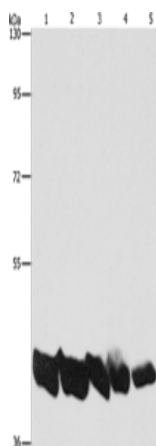
Gel: 10%SDS-PAGE, Lysate: 40 µg; Lane 1-5: A549 cells, hela cells, mouse liver tissue, human liver tissue, hepG2 cells; Primary antibody: 217155(PGK1 Antibody) at dilution 1/850; Secondary antibody: Goat anti rabbit IgG at 1/8000 dilution; Exposure time: 20 seconds
