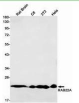
Western blot analysis of RAB22A in rat Brain, C6, 3T3, Hela lysates using Rab22A antibody.
