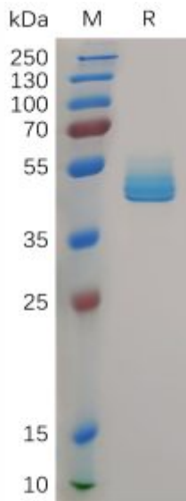
Figure 1. Human CD3D&CD3E Heterodimer Protein, His Tag & hFc Tag on SDS-PAGE under reducing condition.
