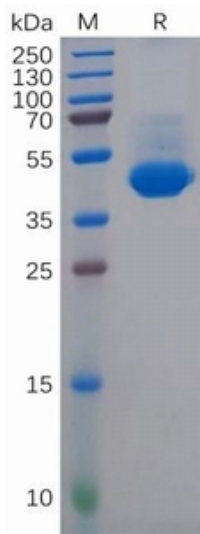
Figure 1. Human NECTIN-4 Protein, His Tag on SDS-PAGE under reducing condition.
